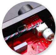
The volume is radjust via the potentiometer ALPS motorized driven by a circuit control by radio frequency remote control
