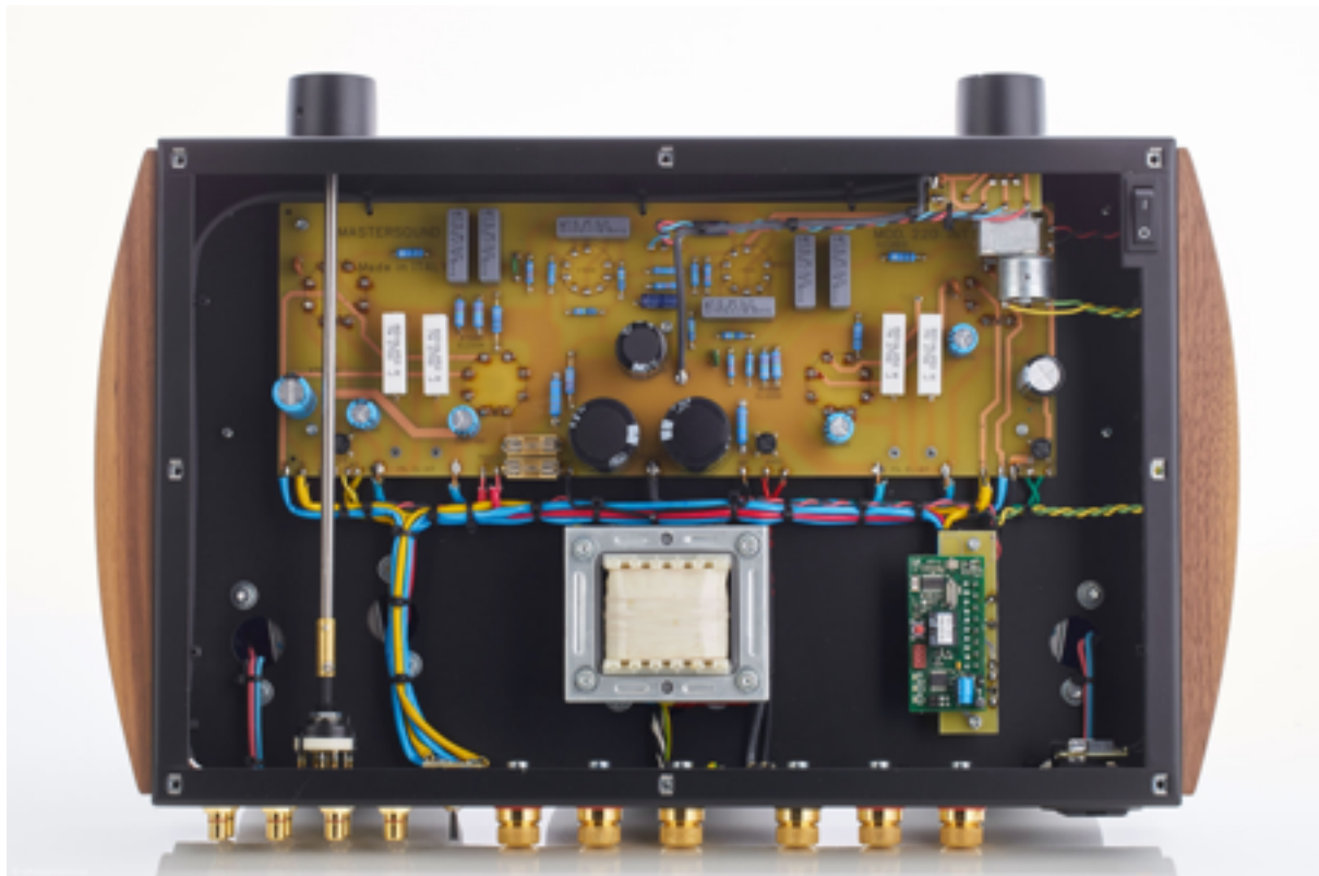
The large screen choke or choke filters high-frequency noise and contributes to the absolutely hum and interference-free reproduction of the Deuventi
