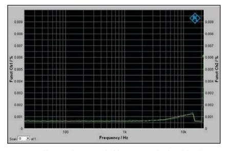
Figure 3: A total harmonic distortion graph of the M1, measured with a Rohde and Schwarz analyzer, shows total harmonic distortion (THD) to be around 0.0006% across most of the audio spectrum. Above 2 kHz, there's a gradual rise to around 0.0025% at 15 kHz, dropping back to 0.0006% between 15 and 20 kHz. (Image courtesy of Bricasti Design, Ltd.)
