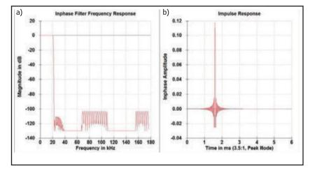
Figure 1: The frequency (a) and impulse (b) responses of a brick-wall, linear-phase filter are shown for a sampling frequency of 44.1 kHz. Pre-ringing, a performance limitation of linear-phase filters, can be seen in the impulse response. (Image courtesy of Bricasti Design, Ltd.)
