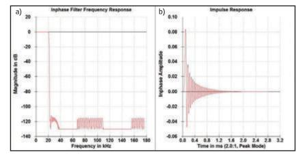
Figure 2: The frequency (a) and impulse (b) responses of a brick-wall, minimum-phase filter are shown for a sampling frequency of 44.1 kHz. Note the absence of pre-ringing in the impulse response. This is a major performance advantage of minimum-phase filters. (Image courtesy of Bricasti Design, Ltd.)
